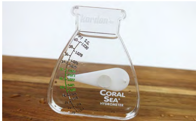
Image shows an example of a swing arm hydrometer by Coral sea.
